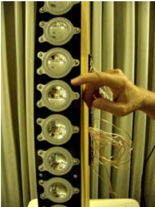
Fig. 14. Close up of the front of the large-driver array of Fig. 13 with the author's hand pointing to one of the drivers. Wiring of the array was in progress.
