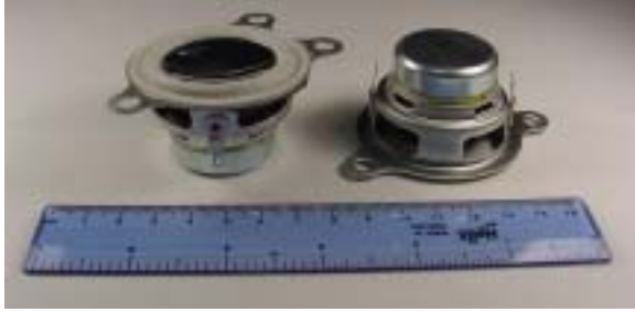
Fig. 11. Photo of the 57 mm (2.25") driver used in the large-driver CBT array. The ruler is a 15 cm (6") long.
