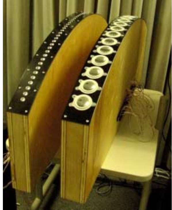
Fig. 17. Oblique side views of the large-driver and small-driver arrays. Wiring is in progress.
