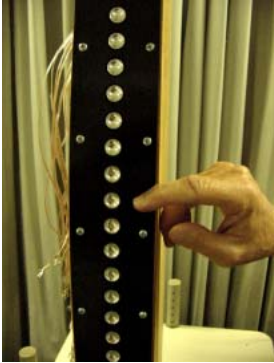
Fig. 16. Close up of the front of the small-driver array of Fig. 15 with the author's hand pointing to one of the drivers. Wiring of the array was in progress.
