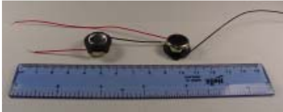
Fig. 12. Photo of the 17.8 mm (0.7") diameter driver used in the small-driver prototype CBT array. . The ruler is a 15 cm (6") long.
