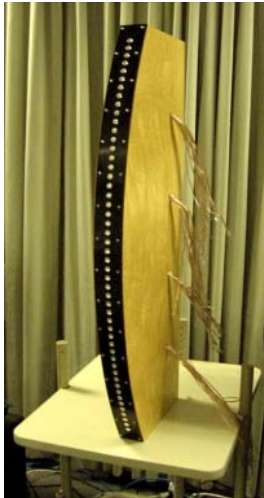
Fig. 15. Photo of the small-driver 60°-wedge-angle 1-m-high prototype array. The array uses 50 each 17.8 mm (0.7") wide-band miniature transducers spaced at 21.2 mm (0.835") center to center. Wiring had not been completed at the time of the photo.
