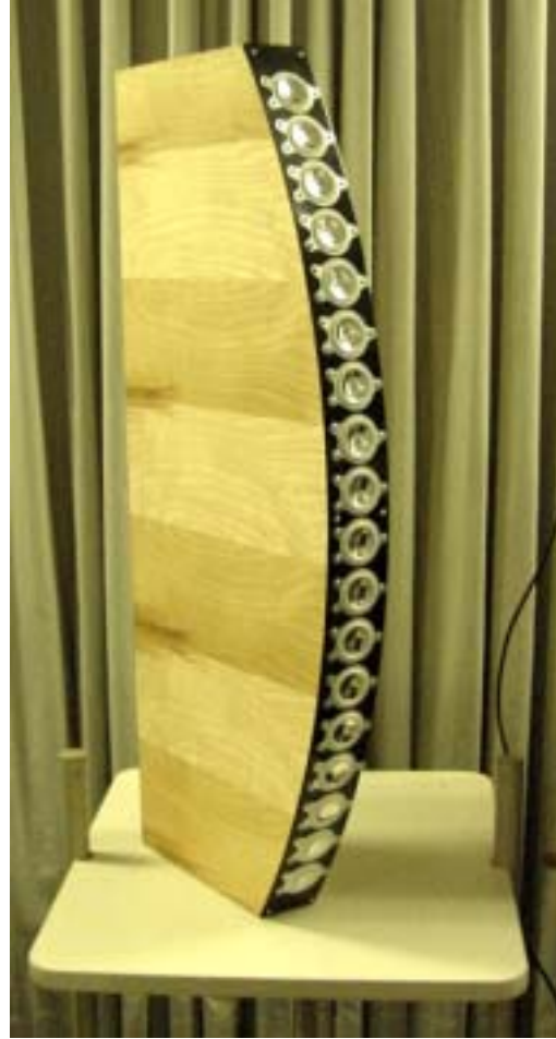
Fig. 13. Photo of the large-driver 60°-wedge-angle 1-m-high prototype array. The array uses 18 each 57mm (2.25") wide-band miniature transducers spaced at 59 mm (2.32") center to center.
